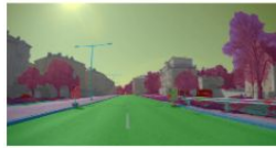
(a) Semantic segmentation results using our modified EfficientNet [18].
