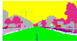
(c) Lidar point clouds (white points) overlaid on the segmented curb pixels.
